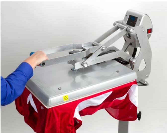
*Note: Please be aware after time is complete, gas shocks will automatically release the platen into the UP position.*
