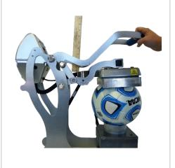
**4.** Align the transfer material on the ball to be printed.
