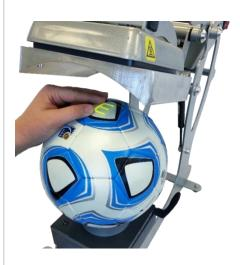
**5.** Lower and lock the handle to print. The timer will count down and automatically raise the heater when the press cycle is complete. When the handle lifts, the timer will re-set and you are ready for the next application.
