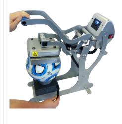
**3.** Using the handle to raise or lower the Ball Mount will adjust print pressure. Most balls will print well with about 2in of space between the Electromagnet and the steel plate on the handle.
